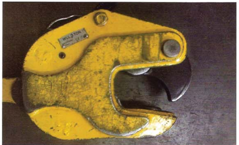
The plate lifting clamp that failed. It has no manufacturer marking or any traceable specification on it
